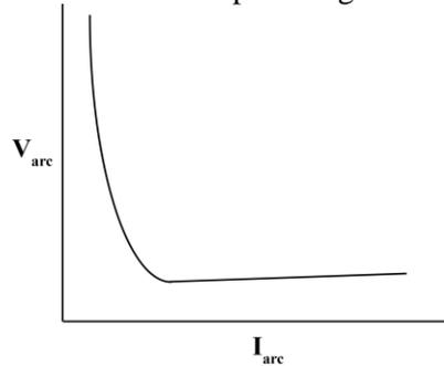
**Fig.2.** Arcing voltage and current characteristic
